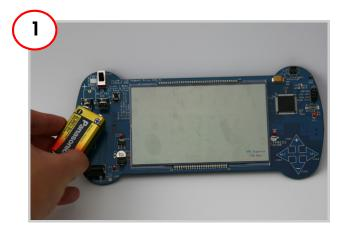
1. Connect 9V battery to board and set the switch to ON.
