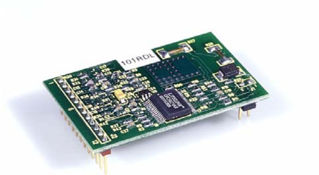
Figure 2. LITELINK III Evaluation Board, Secondary (Bottom) View
