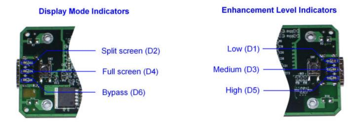
If at any time the hardware detects no valid video source connected at its input, it will for a period of approximately 15 seconds flash the Full Screen display mode indicator, and no video will be present at the output connector. Following this period, if there remains no valid video source at the input, the unit will enter "sleep" mode, in which all indicators are OFF and the output is inactive.
