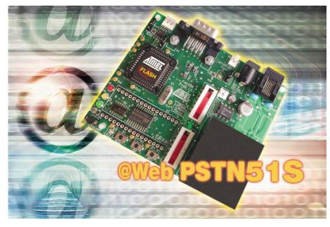
The @Web PSTN51S kit allows the user to evaluate the full range of options available for integrating TCP/IP software into Atmel<sup>®</sup> C51 Flash Microcontrollers.
