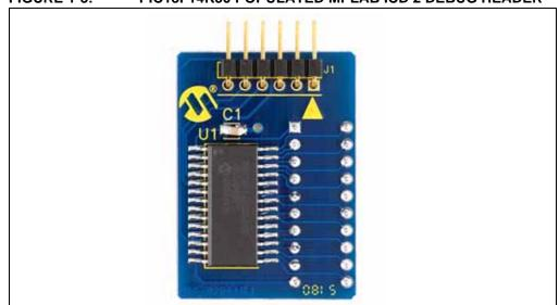
FIGURE 1-3: PIC18F14K50 POPULATED MPLAB ICD 2 DEBUG HEADER
