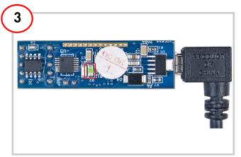
Connect the USB A to Mini B Cable and the bridge to PC. LED D2(green) lights up.
