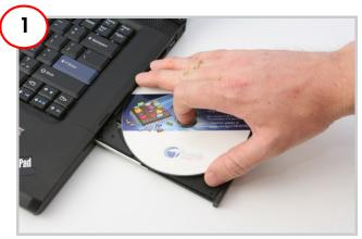
Insert I2C-USB Bridge Kit CD. Install kit contents, PSoC Designer, PSoC Programmer and Bridge Control Panel.
