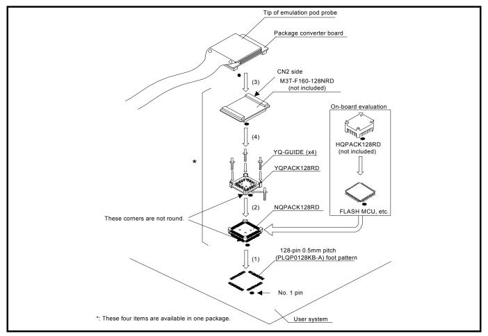
Figure 2.16 Connecting to a 128-pin 0.65mm pitch foot pattern
