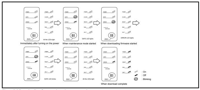
Figure 2.5 Downloading firmware in maintenance mode
