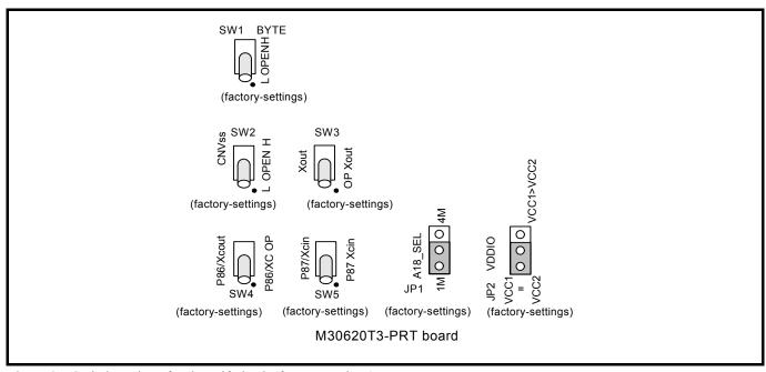
Figure 2.7 Switch settings for the self-check (factory-settings)
