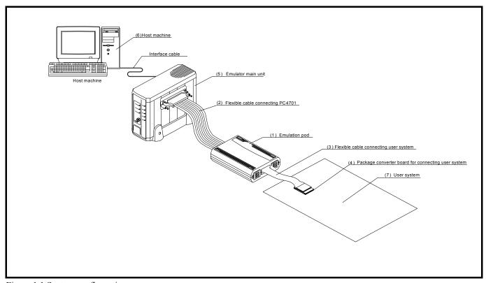
Figure 1.1 System configuration
