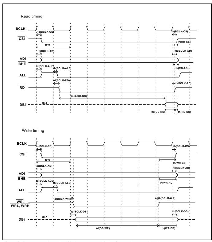
Figure 4.1 Memory expansion mode and microprocessor mode (3 wait, accessing external area)
