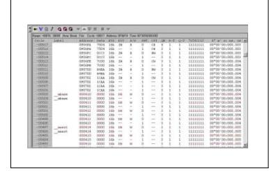
4) Trace Window (Disassemble mode display)
