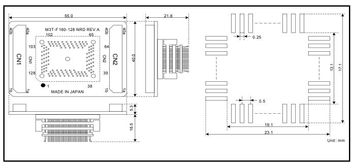
Figure 4.13 External dimensions and a sample foot pattern of the M3T-F160-128NRD
