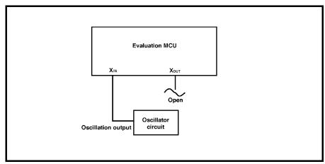
Figure 2.22 External oscillator circuit
