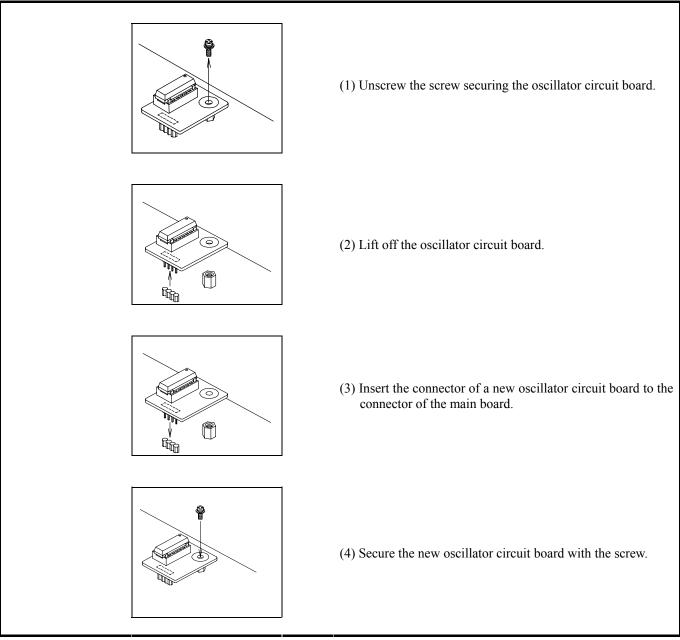
Figure 2.19 Replacing oscillator circuit boards
