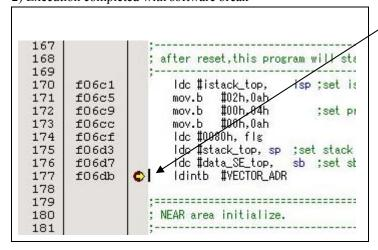
The cursor stops in the position where the software break was set up. The statement in which the software break was set up is not executed.
