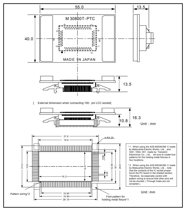
Figure 4.9 External dimensions of the M30800T-PTC
