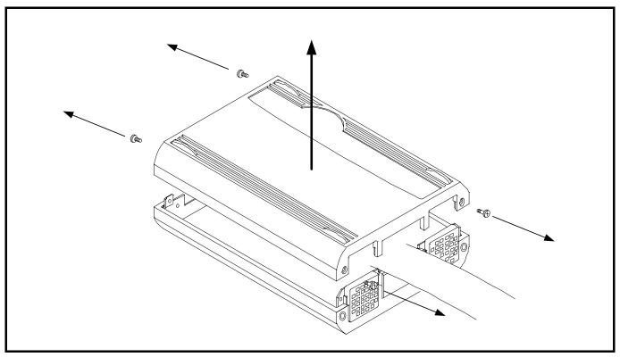
Figure 2.17 Removing the upper cover
