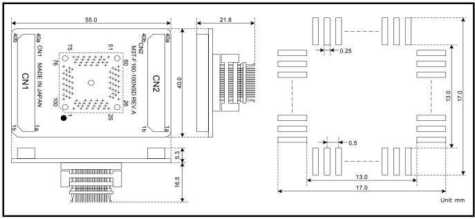
Figure 4.12 External dimensions and a sample foot pattern of the M3T-F160-100NSD
