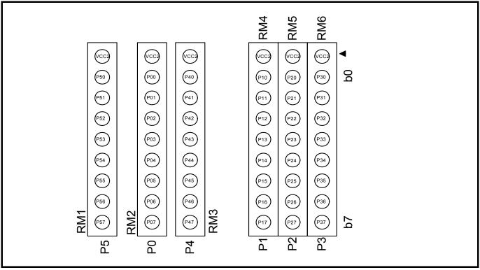
Figure 2.24 Position for mounting network resistors for pullup
