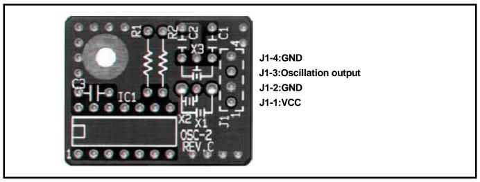
Figure 2.20 External view of the OSC-2 oscillator circuit board and its connector pin positions
