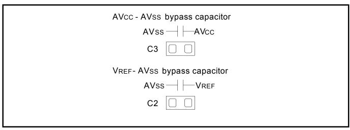
Figure 2.25 Foot patterns of bypass capacitors for A/D converter
