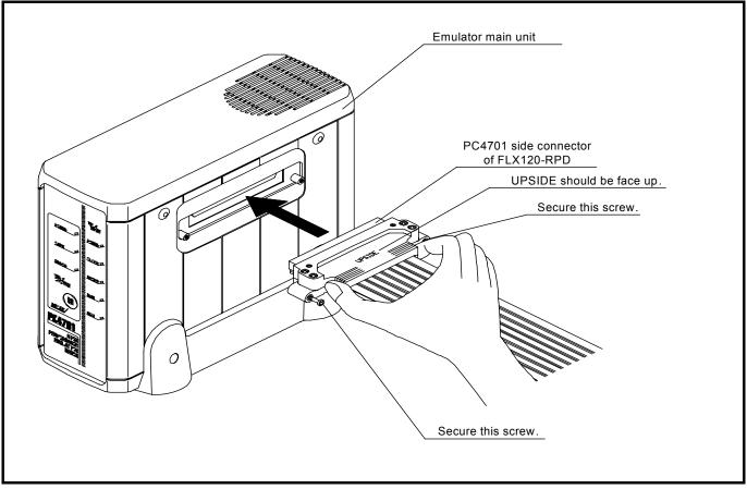
Figure 2.2 Connecting the FLX120-RPD to the PC4701
