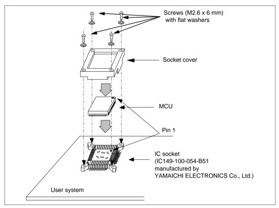
Figure 8 Installing MCU to User System
