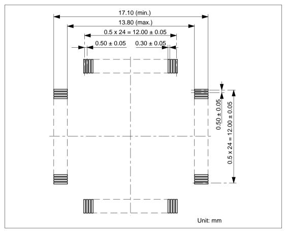
Figure 5 Recommended Dimensions for Mount Pad
