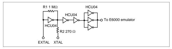
Figure 9 Oscillator Circuit
