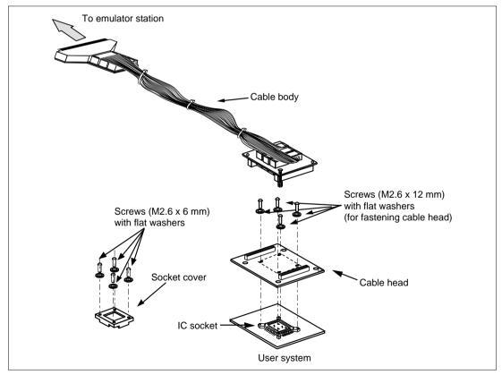
Figure 1 HS2628ECH61H User System Interface Cable
