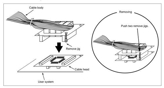
Figure 4 Fastening Cable Body
