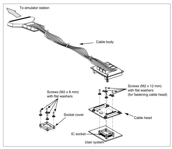
Figure 1 HS2633ECN61H User System Interface Cable
