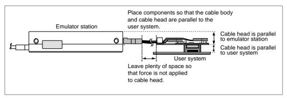
Figure 10 User System Interface Cable Location Example
