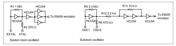
Figure 9 Clock Oscillator Circuits
