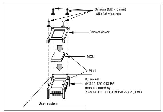
Figure 8 Installing MCU to User System
