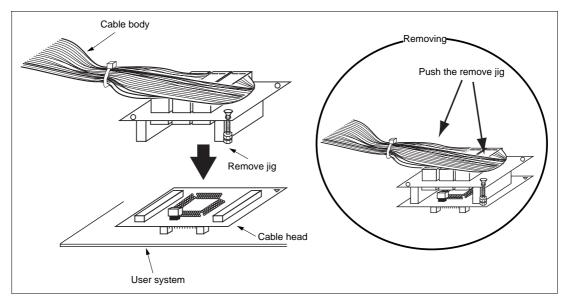
Figure 4 Fastening Cable Body
