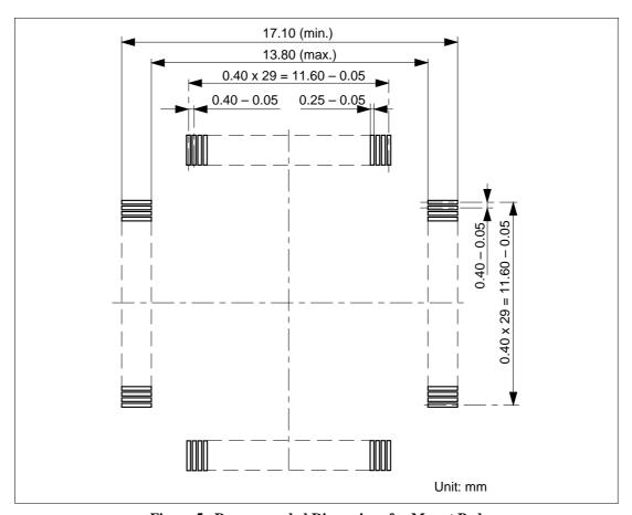
Figure 5 Recommended Dimensions for Mount Pad
