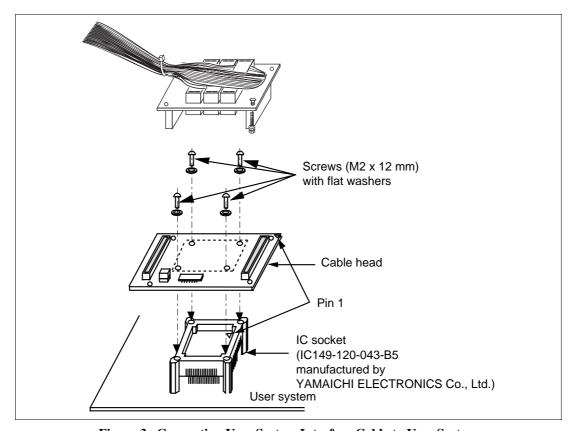
$Figure \ 3 \quad Connecting \ User \ System \ Interface \ Cable \ to \ User \ System$
