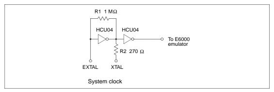
Figure 9 Oscillator Circuit
