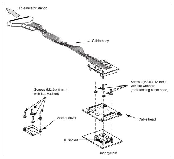
Figure 1 HS2138ECN61H User System Interface Cable
