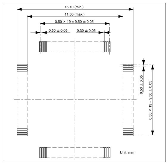
Figure 5 Recommended Dimensions for Mount Pad
