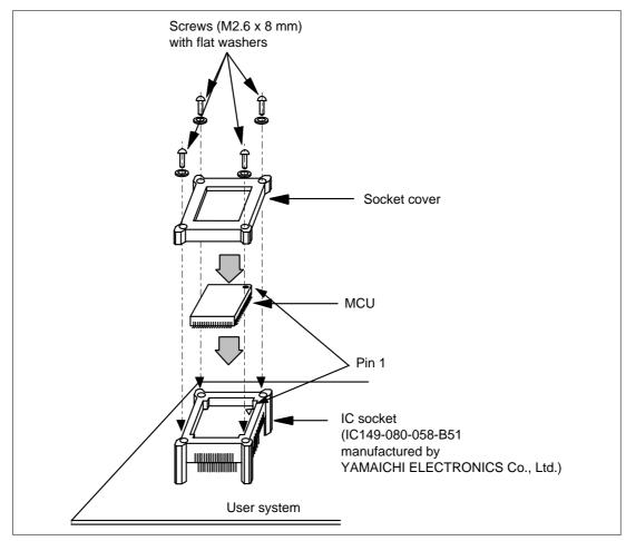
Figure 8 Installing MCU to User System
