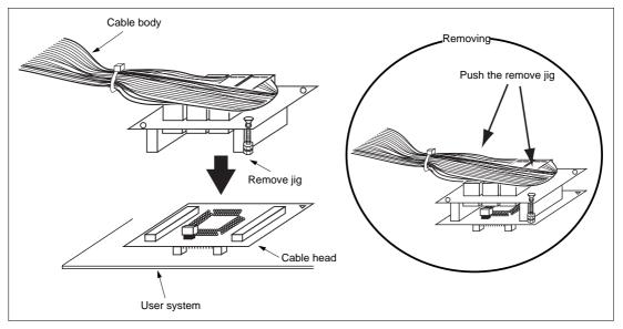
Figure 4 Fastening Cable Body
