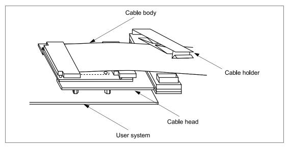
Figure 4 Fastening Cable Body
