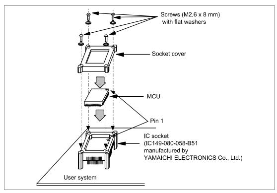
Figure 8 Installing MCU to User System
