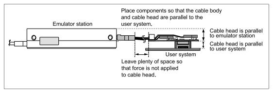
Figure 9 User System Interface Cable Location Example
