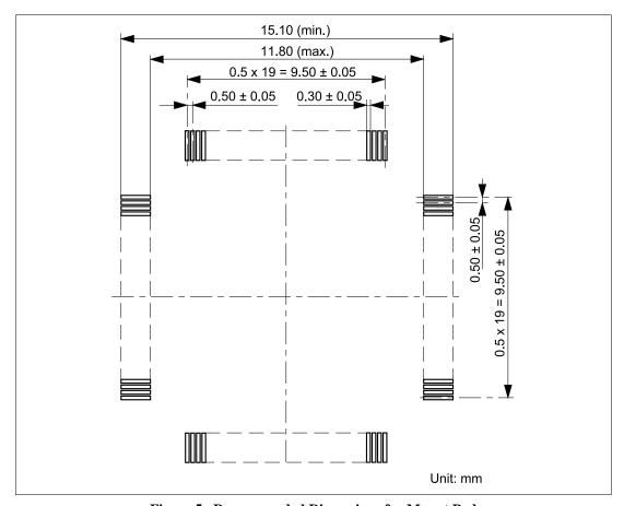
Figure 5 Recommended Dimensions for Mount Pad
