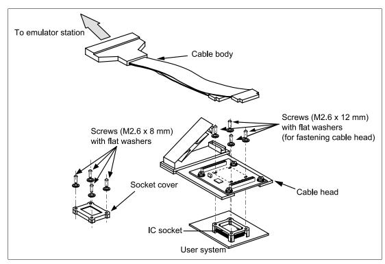
Figure 1 HS2128ECN61H User System Interface Cable
