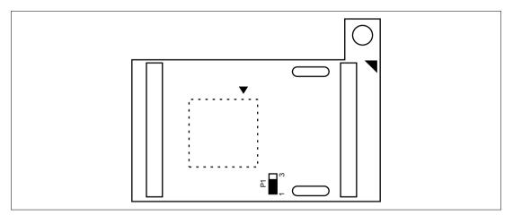
Figure 10 P1 Jumper Socket
