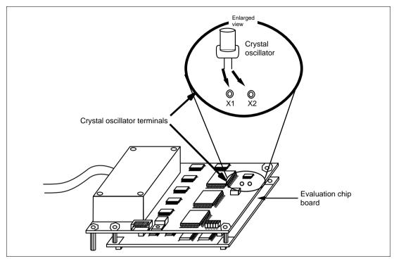
Figure 9 Installing the Clock Oscillator
