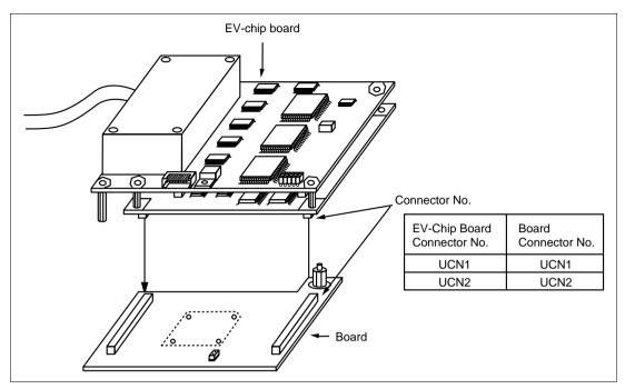
Figure 4 Connecting User System Interface Board to EV-Chip Board
