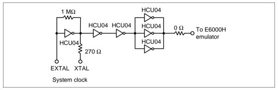
Figure 8 Clock Oscillator
