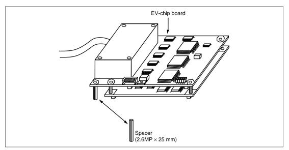
Figure 3 Exchanging the Spacer
