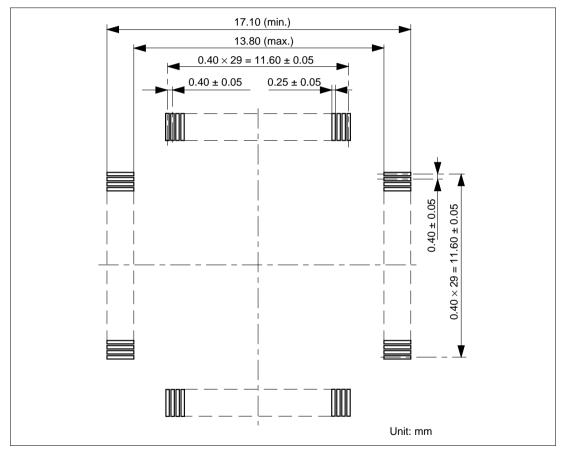
Figure 5 Recommended Dimensions for Mount Pad
