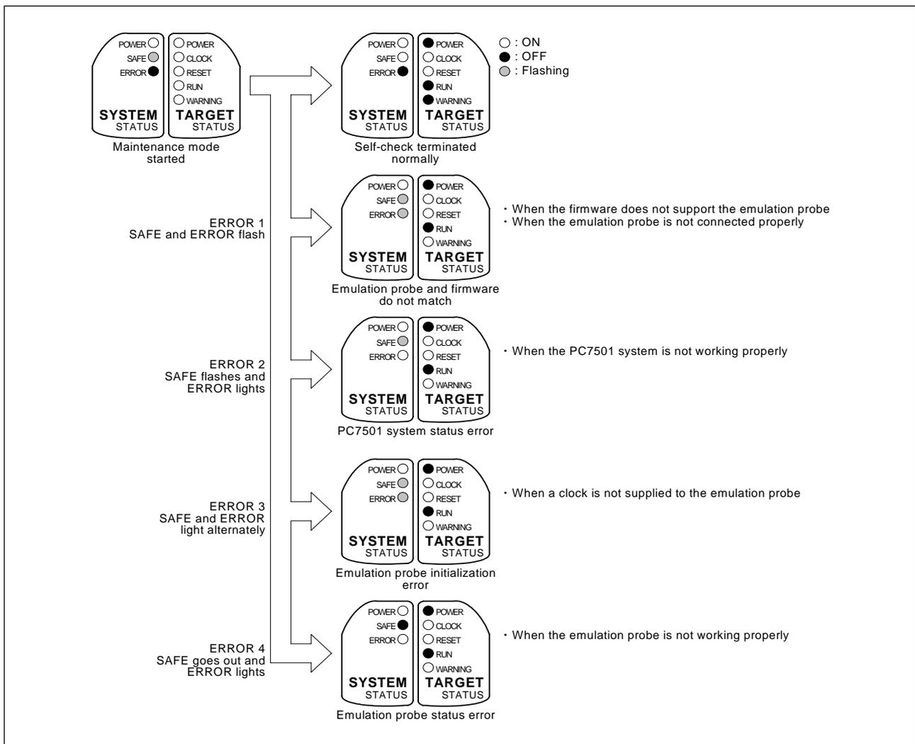
Figure 4.3 LED displays in the self-check
