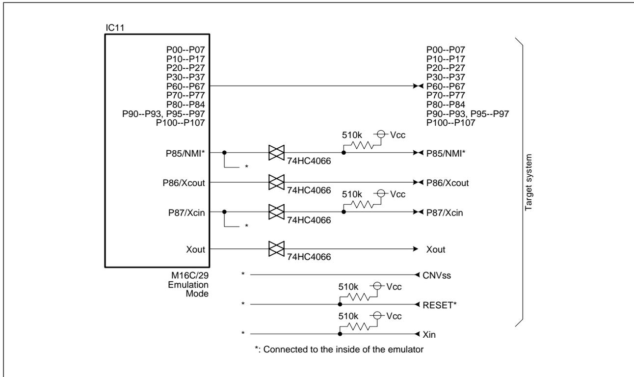
Figure 5.1 Connection diagram
