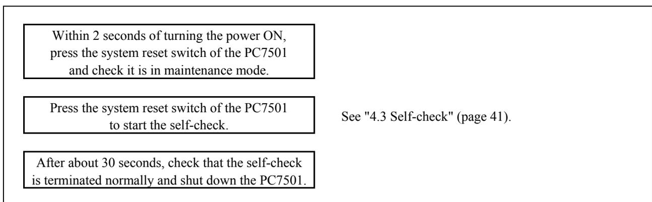
Figure 2.4 Self-check procedure
