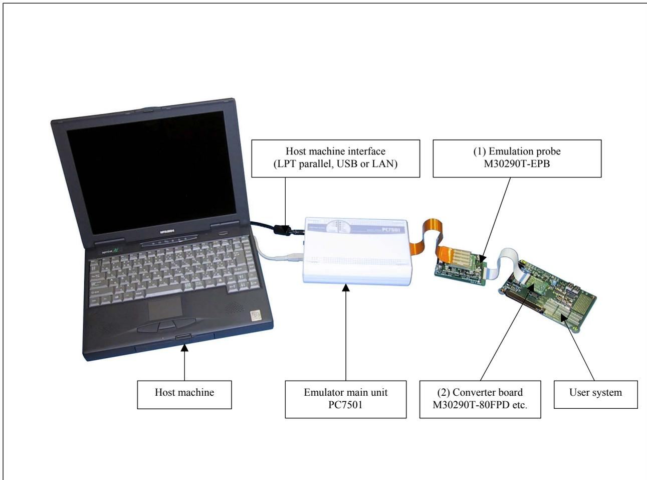
Figure 2.1 System configuration
