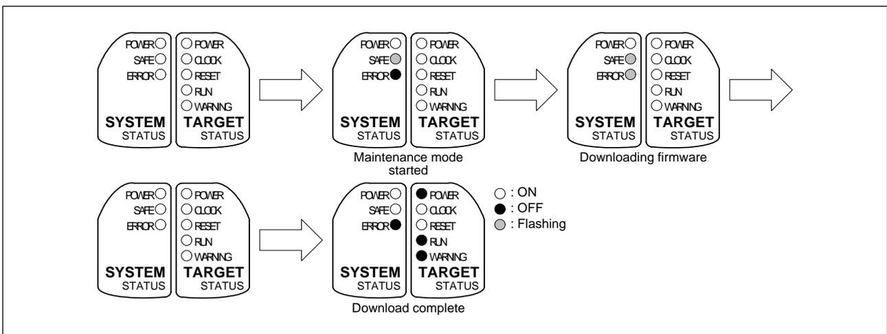
Figure 4.2 LEDs during firmware download
