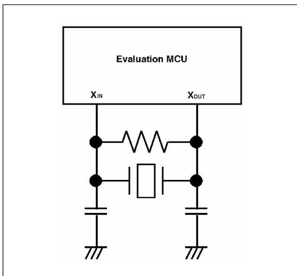
Figure 3.6 Circuit in which oscillation does not occur
