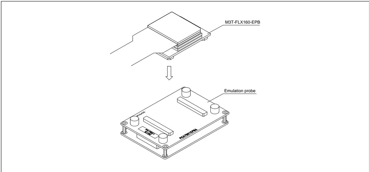
Figure 3.8 Connecting the PC7501 and the emulation probe
