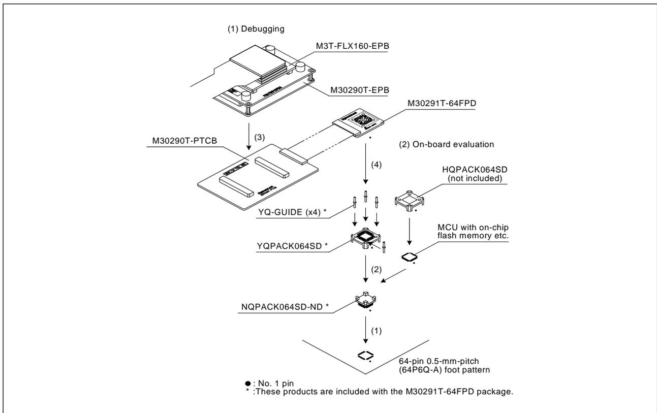
Figure 3.12 Connecting to a 64-pin 0.5-mm-pitch foot pattern
