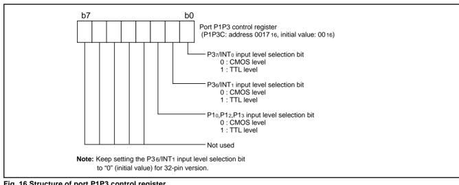
Fig. 16 Structure of port P1P3 control register
