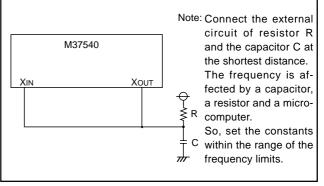
Fig. 47 External circuit of RC oscillation
