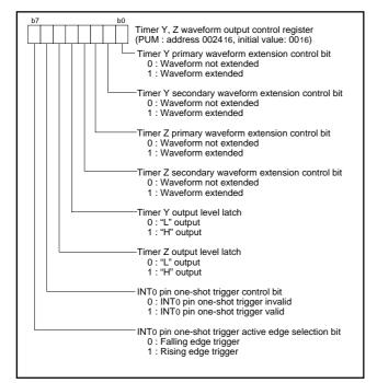
Fig. 26 Structure of timer YZ waveform output control register
