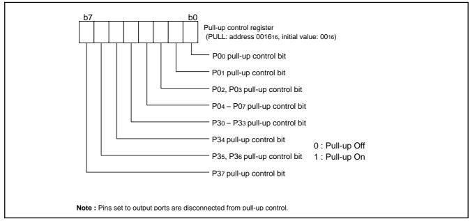
Fig. 15 Structure of pull-up control register
