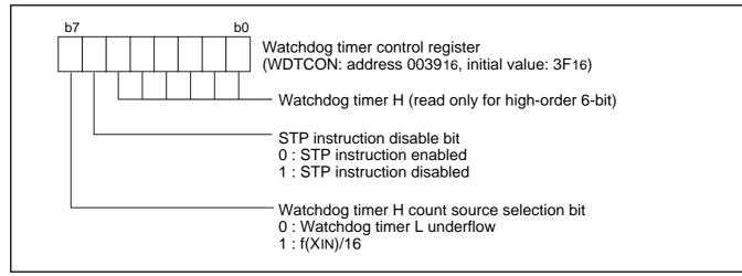
Fig. 42 Structure of watchdog timer control register
