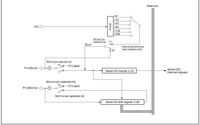
Fig. 36 Block diagram of serial I/O2
