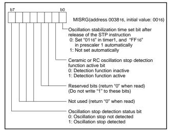
Fig. 50 Structure of MISRG
