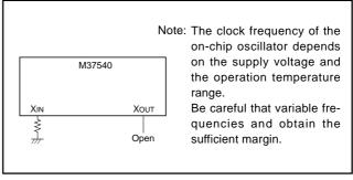
Fig. 49 Processing of XIN and XOUT pins at on-chip oscillator operation
