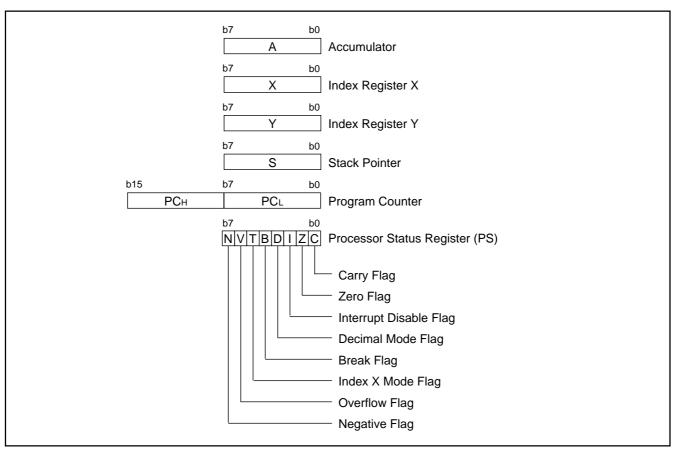
Fig. 9 740 Family CPU register structure
