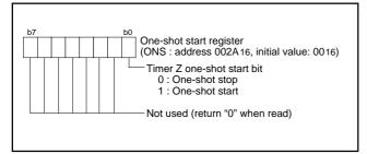
Fig. 27 Structure of one-shot start register
