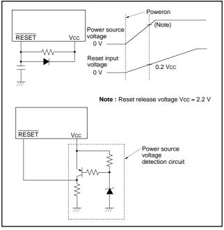
Fig. 43 Example of reset circuit
