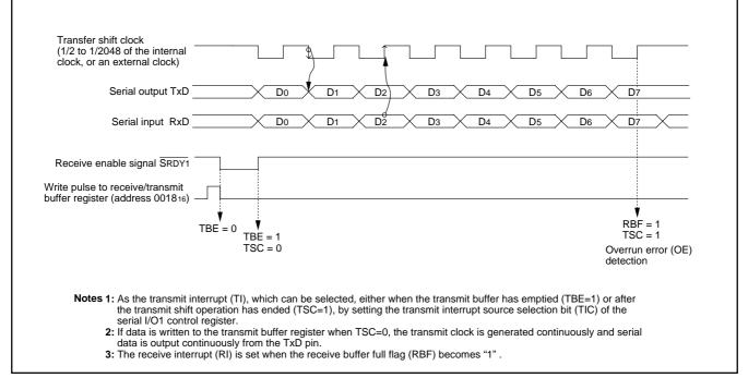
Fig. 31 Operation of clock synchronous serial I/O1 function
