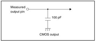
Switching characteristics measurement circuit diagram (General purpose)
