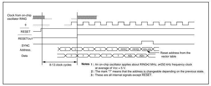
Fig. 44 Timing diagram at reset
