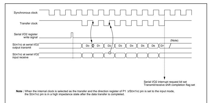
Fig. 37 Serial I/O2 timing (LSB first)
