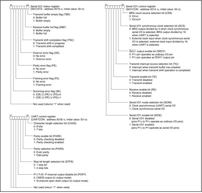
Fig. 34 Structure of serial I/O1-related registers
