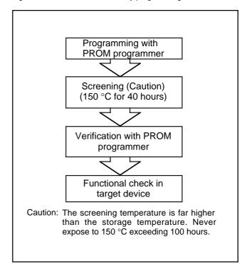
Fig. 54 Programming and testing of One Time PROM version
