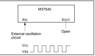
Fig. 48 External clock input circuit
