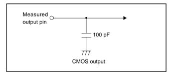
Switching characteristics measurement circuit diagram (General purpose)
