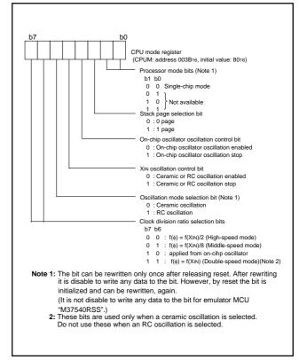
Fig. 11 Structure of CPU mode register
