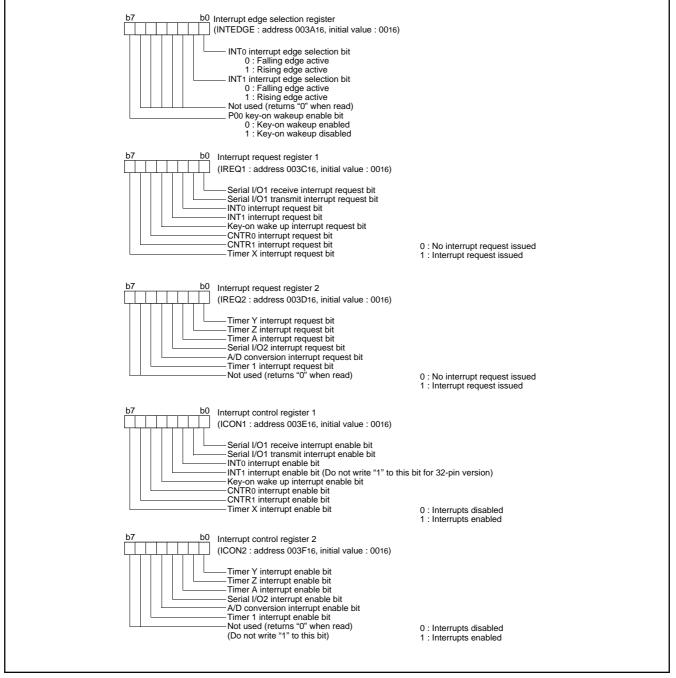
Fig. 20 Structure of Interrupt-related registers
