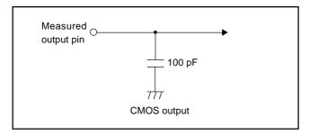
Switching characteristics measurement circuit diagram (General purpose)
