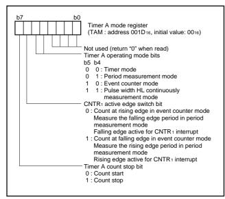
Fig. 22 Structure of timer A mode register
