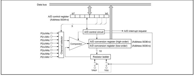
Fig. 40 Block diagram of A/D converter
