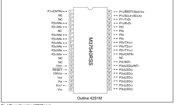
Fig. 4 Pin configuration (42S1M type)
