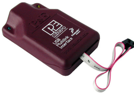
Figure 9-1: P&E's USB Multilink (USB-ML-12 shown)
