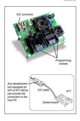
The illustration and photo show one example of ST7-SocketBoard. However, programming sockets vary for the different models of socket boards, depending on package types for the ST7 family that they support.
