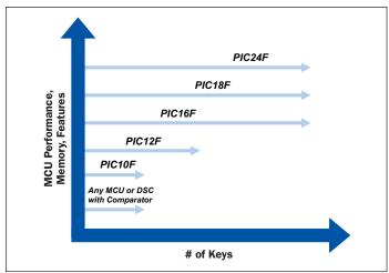
Microchip's Capacitive mTouch Solution offers a number of PIC MCUs to suit the demands of any application from the most basic single-button design using the incredibly small and cost-effective 6-pin PIC10F to the peripheral rich 8-bit Mid-Range and 16-bit microcontroller families.
