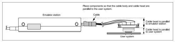
Figure 12 User System Interface Cable Location Example
