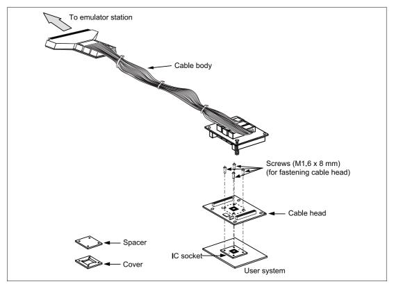
Figure 1 HS2238RECB62H User System Interface Cable
