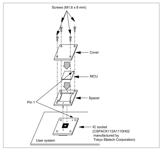
Figure 10 Installing MCU to User System
