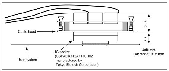
Figure 9 Resulting Dimensions after Connecting User System Interface Cable
