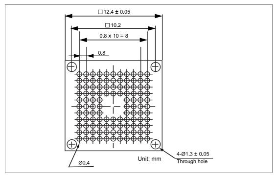
Figure 7 Recommended Dimensions for Mount Pad
