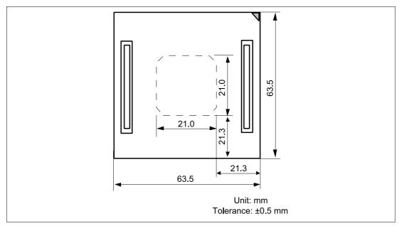
Figure 8 Dimensions for User System Interface Cable Head
