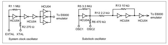
Figure 11 Oscillator Circuit
