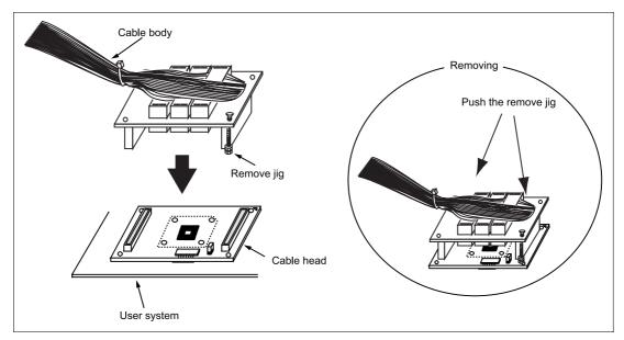
Figure 6 Fastening Cable Body
