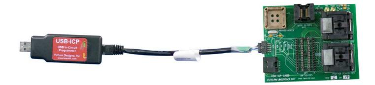
To use the SAB9, it must first be connected to a PC through a USB-ICP with a USB-ICP-LPC9xx cable to P1, as shown above. Or, if you do not have the USB-ICP-LPC9xx, the SAB9 may be connected to the PC with regular Ethernet Patch cable to P2, as shown below. The USB-ICP must then be connected to the USB port on your PC. To learn more about using the USB-ICP, please visit www.teamfdi.com/usb-icp
