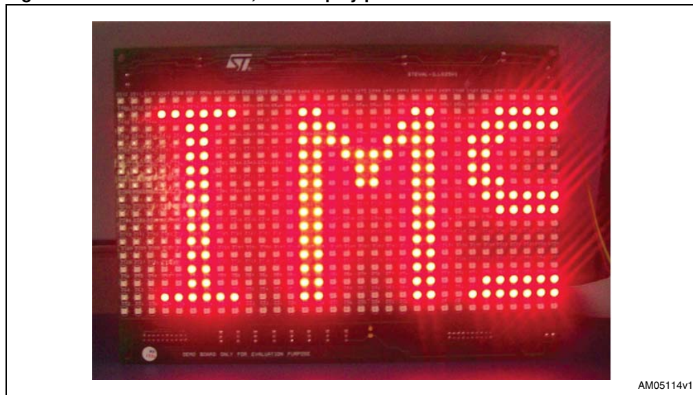
Figure 1. STEVAL-ILL025V1, LED display panel
