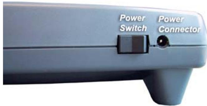
**3.3.8 Power Connector** The Power Connector on the ICE50 system is a standard type with 2.1 mm center tap. Ground should be connected to the center tap. For more information about power requirements and operating conditions see the Power System Description. See Figure 3-7.
