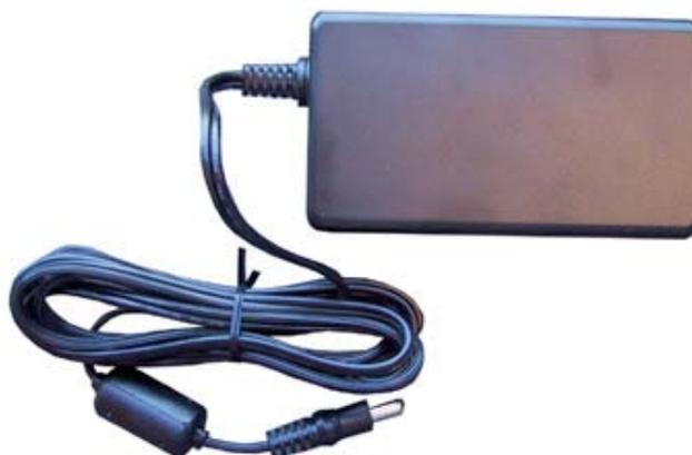
The power supply delivered with ICE50 is dimensioned to meet the requirements of the Emulator. If another power supply is used, it should supply a voltage between 9 and 15 VDC, and a minimum of 20W. It connects to the main unit through a standard connector with 2.1 mm center tap. Ground is connected to the center tap.
