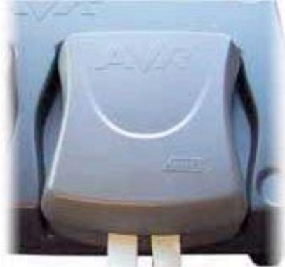
The POD contains all analog and digital logic necessary to emulate the target AVR device. The circuitry is designed to give as close as possible electrical characteristics as the real device. The POD emulates the following functions:
