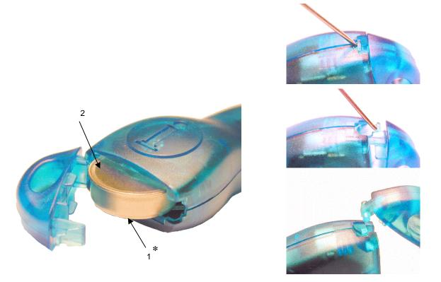
\*Note: The data contact faces down and away from the embossed 'i'. Once the <u>i</u>Button is inserted in the enclosure, snap the end cap over it. The end cap is removed by depressing the release tab with a paper clip, swinging it fully open, and sliding out the hinge.
