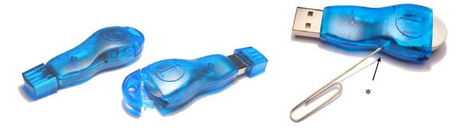
\*Note: To eject an <u>i</u>Button, insert a straightened paper clip into the side access hole of the DS9490B. Push the paper clip in the direction of the <u>i</u>Button. A different <u>i</u>Button can then be inserted. The data contact faces down and away from the embossed 'i'. Before inserting the paper clip disconnect the DS9490B from the USB bus.
