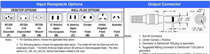
3. Blade Kit is available which will include one each of a EU, UK, and Aust blade. Kit part number is KT1027K. Can be used with (B) version only, to allow blades to be interchanged.
