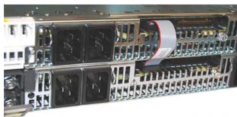
Shelf-to-shelf cable connection (part # CC848848952)
