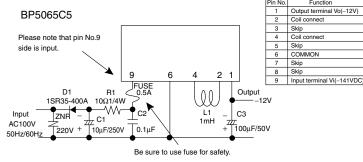
Please verify operation and characteristics in the customer's circuit before actual usage and ensure that the load current does not exceed 200mA.
