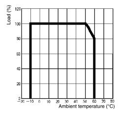
For UL and CSA the maximum temperature is 50% (with derating of 2%°C from 40 °C to 50 °C, only for 40 A model)
