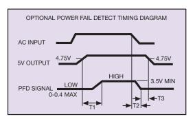
Power fail detect signal 50 ms≤T1≤200 ms T2 will vary with line and load T3≥3 ms Pout: 110 W PFD output is an open collector which will sink ≤40 mA in the low state.
