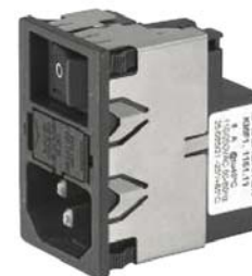
Fig. 15a External filter to reduce conducted emissions of LW models with feature E ( L_1 = L_2 = 1.6\ mH , C_x = 47\ nF , C_y = 2.2\ nF )
