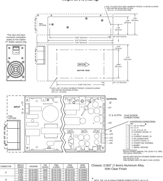
Overall Size: 8.50" x 4.75" x 2.00" (215.9mm x 120.7mm x 50.8mm) Overall Length With Fan: 10.00" (250.4mm) Weight: 2.75 lb (1.25 kg)
