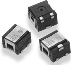
Tyco Electronics are pleased to introduce this tiny (4mm square) multiturn trimmer potentiometer. The 3240 Series is designed with a footprint meeting EIA and other international board layout standards. It is also compatible with all surface mount manufacturing processes. It is ideally suited to small sensors where its 10 turn setability and small size enables it to stand out from most other competitors.
