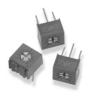
A tiny, fully sealed, professional trimmer offered with a range of pin configurations. The 4275 is available with top or side adjustment. Standard packaging is in tough plastic tubes. The cermet element is very stable and has good setability.
