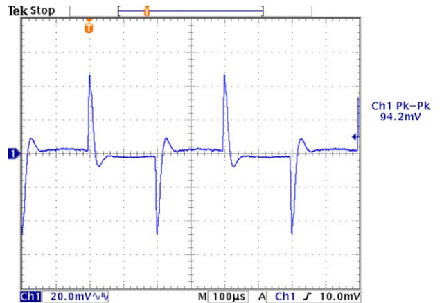
Figure 20. Transient Response without Optimal Voltage Positioning
