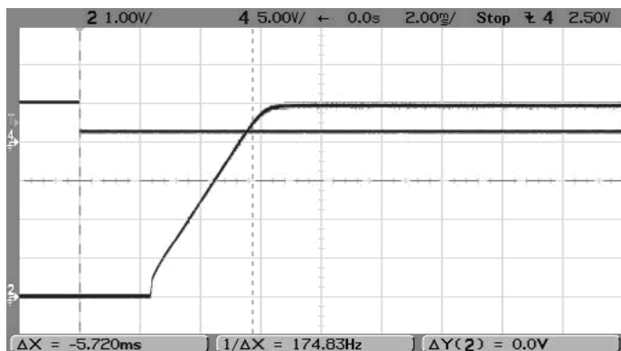
On/Off Enable Delay (Vin=12V, Vout=5.0V, Iout=6A, Load=0) Trace 4=Enable, Trace 2=Vout
