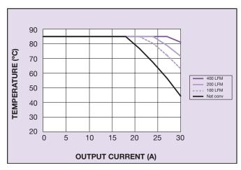
Figure 1 - Safe Operating Area Vin = 3.3 V, Output Voltage = 2.5 V (See Note A)
