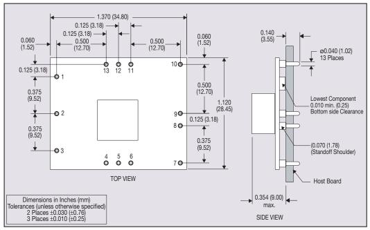
Figure 4 - Plated Through-Hole Mechanical Drawing
