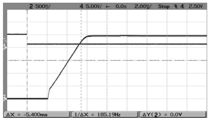
On/Off Enable Startup (V in =5V, V out =2.5V, I out =6A, Cload=0) Trace 4=Enable, Trace 2=Vout
