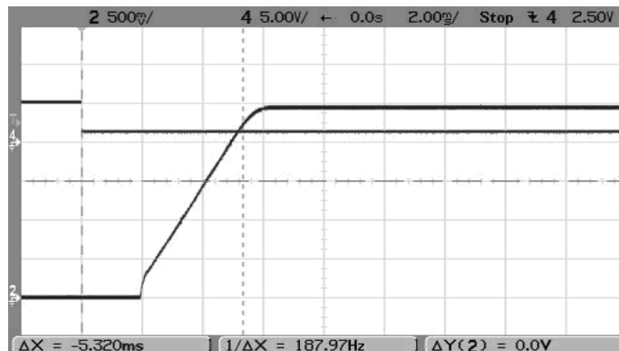
Step Load Transient Response (Vin=5V, Vout=2.5V, Clod=0, Iout=3A to 1.5A) Trace 2=Vout, 100 mV/div. Trace 4=Iout, 1A/div.
