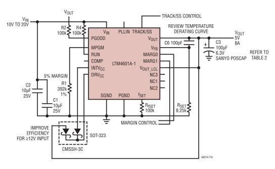
Figure 16. 5V at 8A Design Without Differential Amplifier
