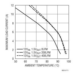
Figure 11. No Heat Sink  $12 V_{\rm IN}$
