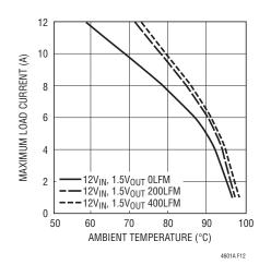
Figure 12. BGA Heat Sink  $12V_{IN}$
