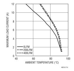
Figure 14.  $12V_{IN}$ ,  $3.3V_{OUT}$ , BGA Heat Sink
