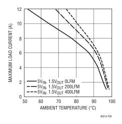
Figure 9. No Heat Sink 5V<sub>IN</sub>
