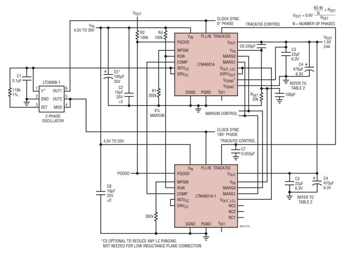
Figure 19. 2-Phase Parallel, 1.5V at 24A Design
