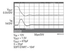
Start-Up, I<sub>OUT</sub> = 12A (Resistive Load)
