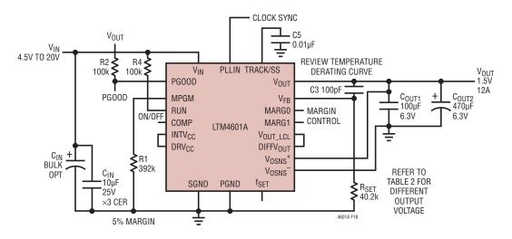
Figure 18. Typical 4.5V-20V<sub>IN</sub>, 1.5V at 12A Design
