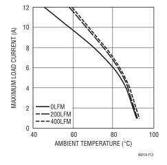
Figure 13.  $12V_{\text{IN}},\,3.3V_{\text{OUT}},\,\text{No}$  Heat Sink
