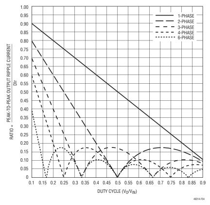
Figure 4. Normalized Output Ripple Current vs Duty Cycle, DIr = V<sub>0</sub>T/L<sub>1</sub>, DIr = Each Phase's Inductor Current
