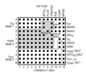
**INTV<sub>CC</sub> (Pin A7, D9):** This pin is for additional decoupling of the 5V internal regulator. These pins are internally connected. Pin A7 is a test pin.
