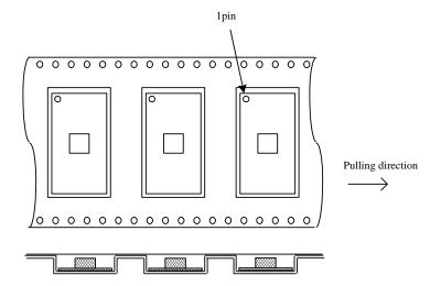
The module is located such as parts in upper side and PCB in lower side.
