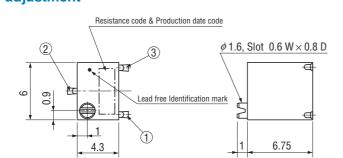
Unless otherwise specified, tolerance :  $\pm$  0.3 (Unit: mm)
