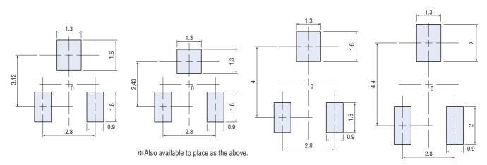
Note) The zero point is the center of mounting.
