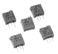
The Model 64 is a small size trimmer - 3/8" x 3/8" x 3/16" - answering PC board mounting requirements. Five versions are available which differ by the position of the control screw in relation to the PC board plane and by the spacing of the terminals. Excellent operational stability is provided by the use of a cermet element.
