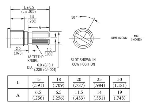
This change affects Model PDB181 and PDB182 with knurled shaft only. The shaft material will change from aluminum to zinc-die cast. In addition, the rear cover will be tin-plated rather than zinc-plated to allow customers to solder to the rear cover. Two new shaft lengths will be available: 15 mm and 18 mm. There are also a few minor dimension changes to the anti-rotation lug and terminals that do not affect fit. Please see the Model PDB18 data sheet for detailed dimensions.
