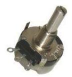
53 Series Industrial Potentiometer, Conductive Plastic Element, Solder lug Terminals, 2 W Power Rating, 2 kOhm Resistance Value
