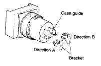
To produce continuous sounds, attach the bracket to the case guide so that the triangle on the bracket faces direction B.
