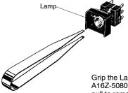
Grip the Lamp with the A16Z-5080 Extractor and pull to remove.
