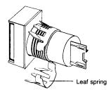
Insert the buzzer assembly into the hole on the mounting panel from the front.
