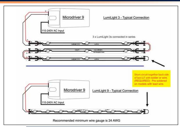
Maximum current input 350mA Maximum power consumption 1.2W per LED for White / Blue / Green 1.0W per LED for Red / Amber
