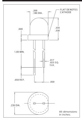
The Ultrabright CMD3X50 Series LED lamp provides exceptional brightness in a very narrow viewing area, in a clear tinted non-diffused package making them excellent for small area backlighting. A pale tint aids in identification. The High Efficiency Red and Yellow lamps are produced with GaAsP/GaP and the High Efficiency Green lamp is produced with GaP/GaP. All feature an 80 mcd minimum luminous intensity.
