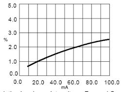
Relative Luminous Intensity vs Forward Current
