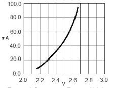
Forward Current vs Forward Voltage
