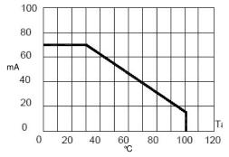
Maximum Forward DC Current vs Ambient Temperature
