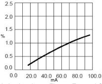
Relative Luminous Flux vs Forward Current
