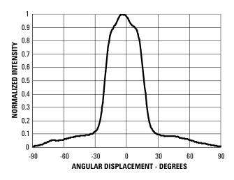
Figure 5. Representative Spatial Radiation Pattern of the — minor axis
