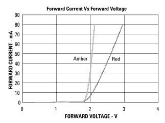
Figure 2. Forward Current vs. Forward Voltage
