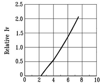
Fig.3 Relative Luminous Intensity vs. Applied Forward Voltage
